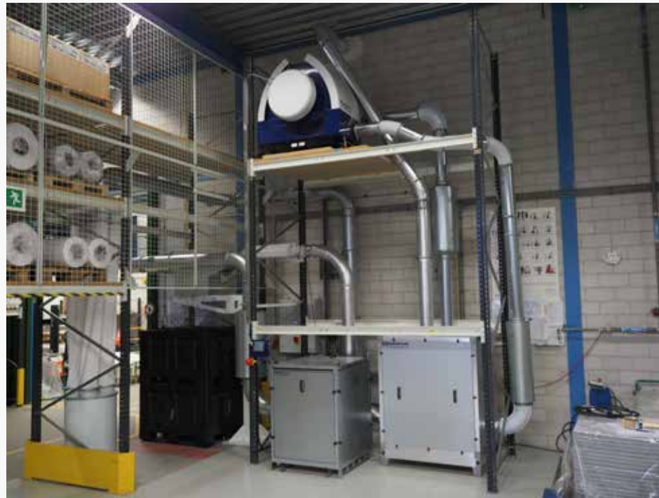
The MultiAir® blower is placed on a frame to optimize floor space
