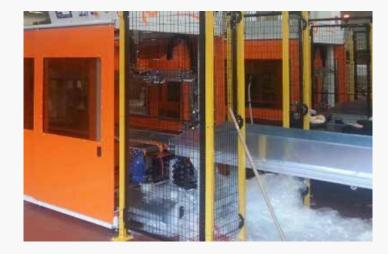
• In the old conveying solution, plastic wrap often ended below the belt before being pick up and was manually transported to the waste container.
