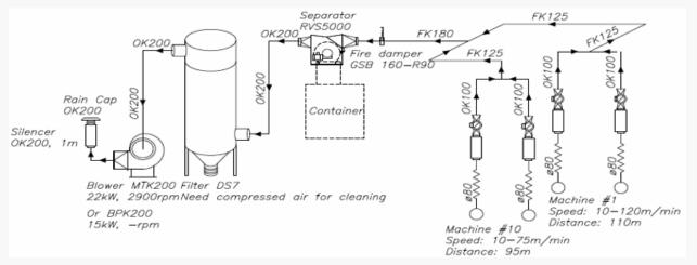
The drawing shows two production machines as the system is prepared for an additional machine to be installed in the future
