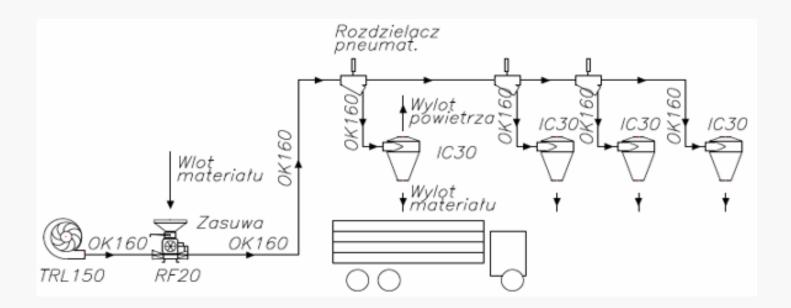
The Kongskilde solution consisted of a TRL100 blower with RF40 Rotary Valves. This system secures a dynamic form of transport of the material that obtains an adequate material yield with use of the TRL 100 blower as well as a vigorous discharge of the pomace directly in the lorries
