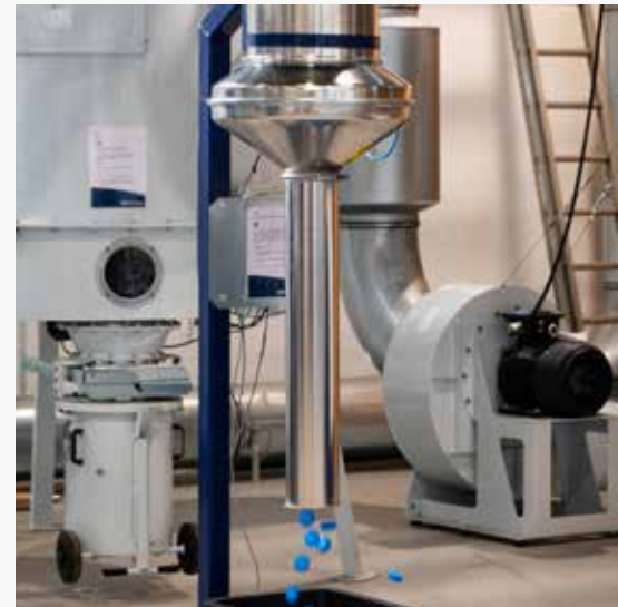
The CVL units separate components and air
