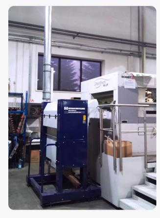
The Kongskilde MultiDicer efficiently cuts thick paperboard into small, uniform pieces for easy pneumatic transport, ideal for removing die-cut skeletons and improving waste handling in packaging production.
