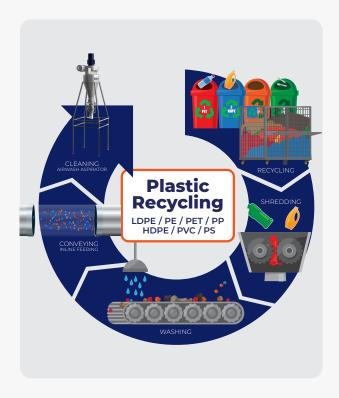
The AirWash aspiration system is an effective solution for separating and cleaning plastic pellets and granules for recycling. Unwanted fines and dust are removed and collected, ultimately improving the quality of reusable materials.
