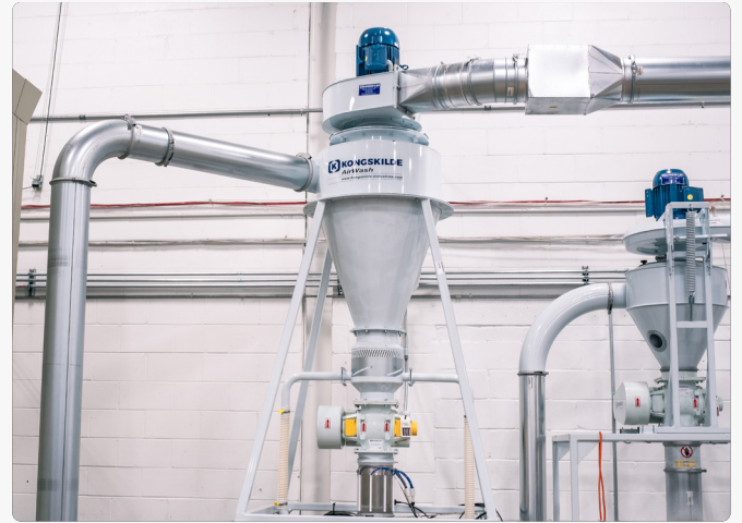
The AirWash pulls regrind from the granulator under vacuum, removing dust and fines through a two-stage cyclonic and anti-static process.
