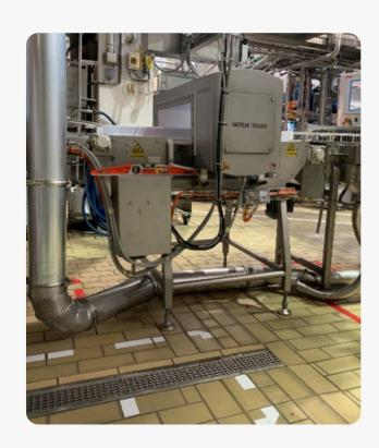
**Individual conveying lines** from each production machine make it possible to keep different waste materials/colours separated.
