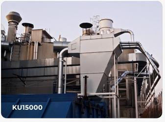
**KU Static Separator** directs bulk materials into a stationary compactor, baler, or container, while the conveying air is efficiently expelled, enabling clean, efficient waste collection.
