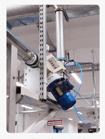
The Kongskilde MultiCutter shreds film scraps directly at the source, enabling smooth, uninterrupted transport through the system.
