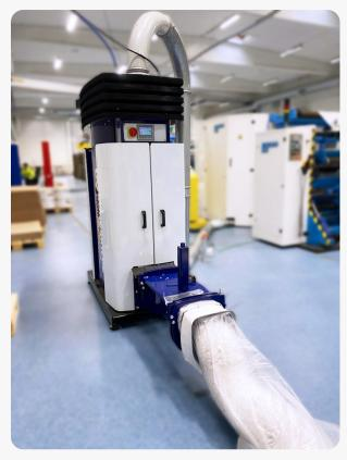
Designed for efficient and continuous trim collection, the **CUC**'s compact design and endless bag system ensure seamless operation with minimal maintenance and easy waste handling.
