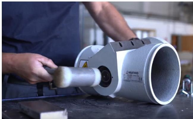
11 - Pull out the rotor. When removing the rotor, be careful not to cut yourself on the sharp knives. The edges are fragile, make sure they dont hit the housing during removal.
