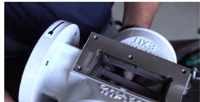
19 - Install the fixed knife with adjustment plate.
