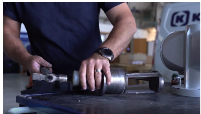
13 - Insert the smallest lock ring on the opposite side of the motor flange.
