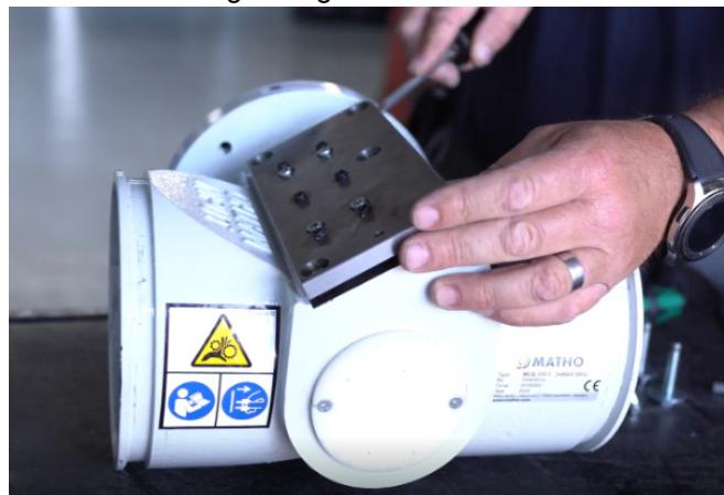
6 - Next remove the screws from the top of adjustment plate. Leave the pinion screws in.
