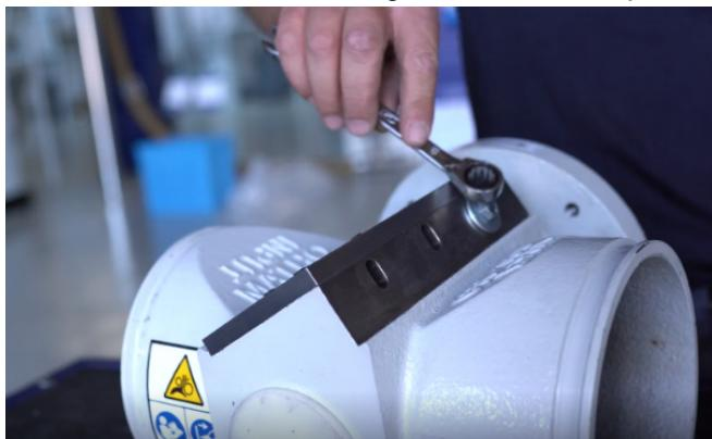
5 - When all screws are removed, carefully lift up the complete assembly with fixed knife and knife adjustment plate. It might be needed to use a flat head screw driver or similar in order to lift it out. Be careful of the sharp blade.
