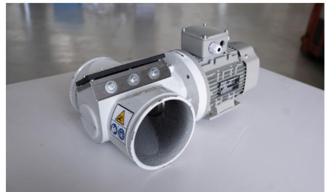
2 - Remove the motor, by loosing the 4 screws on the motor flange. Remove the plastic coupling part.
