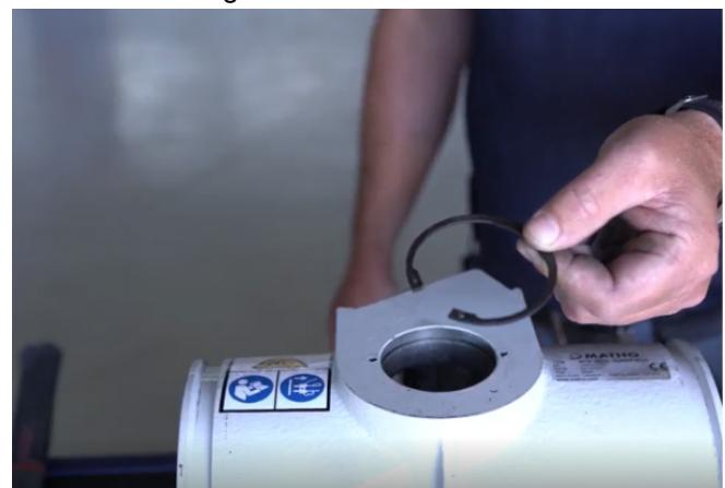
14 - Carefully install the bearing housing, and insert the rotor. Make sure the rotor does not strike the housing, the knives are fragile.
