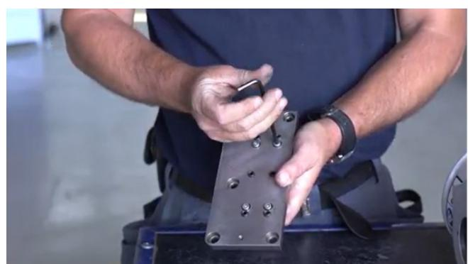
7 - The fixed knife is now separated from the adjustment plate.
