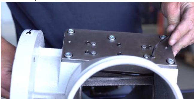
2 - Now tighten the retaining screws to lock the fixed knife in place.
