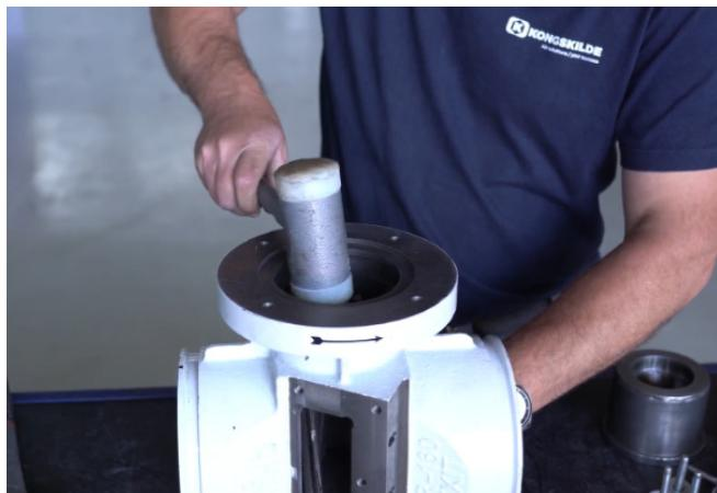
16 - The rotor is fully inserted when the big lock ring can be reinstalled. When lock ring is inserted, check that the rotor can rotate without resistance. If resistance is felt, use the plastic mallet and force the rotor back towards the big lock ring. Now it should move freely.
