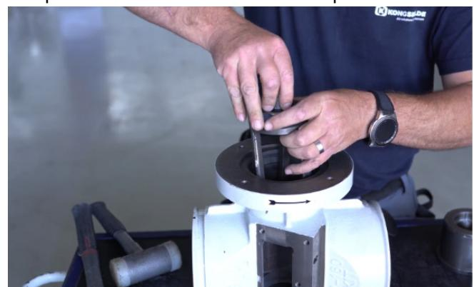
15 - Tap the rotor with a mallet, to fully insert the rotor.
