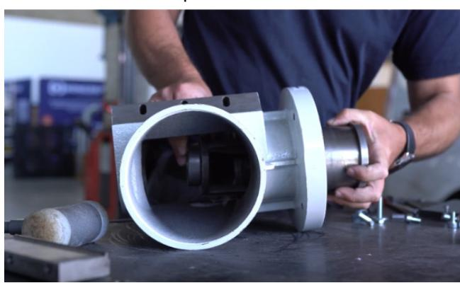
12 - Now remove the rotor from the bearing housing, by means of a plastic or rubber mallet or regular hammer on a mandrel.
