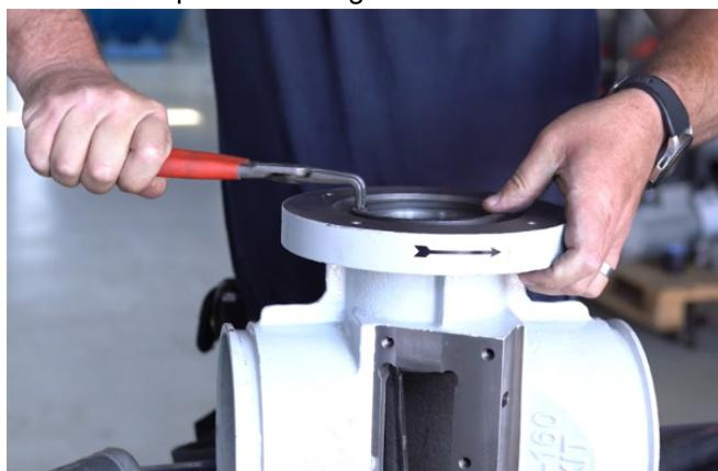
17 - Mount the fixed knife in the knife adjustment plate.
