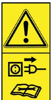
Always disconnect the power to the trim handler before repair and maintenance and ensure that it cannot be started by mistake.
