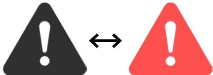
If a fault occurs in the frequency converter, this icon in the top left corner will flash, changing from black to red. The error messages are sent from the frequency converter control directly to the operator panel. By pressing the icon, it is possible to read and reset the fault by pressing Reset Faults. This can only be done as user Admin, and only if the fault can be corrected by resetting.
