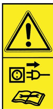
Piping must not be removed while the CVL is in operation. Wait until compressed air and electricity has been disconnected.
