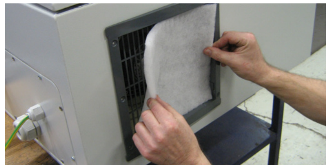
3 - remove the filter, and clean if necessary. Reinstall in reverse order.
