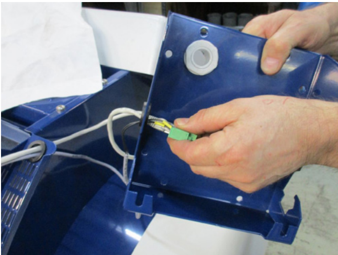
5 - The cable relief in the panel's bracket is loosened, the wires are pulled out of the bracket and out of both holes in the blower's end plate, and guided down the left side of the blower.
