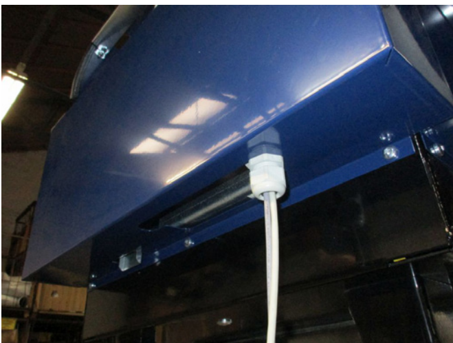
6 - Both wires are led through an M25 cable relief (not included), that must be fitted at the front or back of the blower's base frame, taking into account the operator panel's new location.
