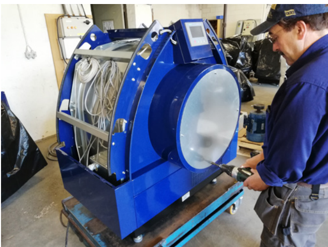
3 - remove the motor cover by removing 4 screws, and put the cover aside
