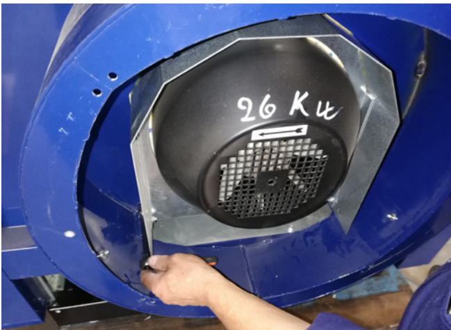
8 - loosen 2 nuts, 1 in each side
