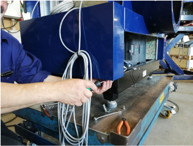
13 - also remove the 3 lower screws holding the blue side panel, and put the panel aside
