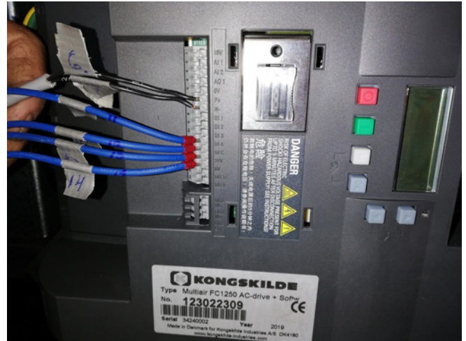
34 - reconnect the AC drive control wires according to the tape markings, by depressing the release buttons with a straight edge screwdriver. Refit all cable ties.
