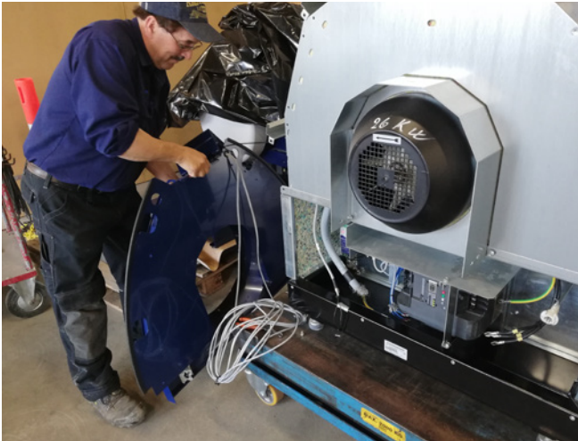
19 - put the blowers end plate aside, ensuring that the cables to the operators panel are not damaged
