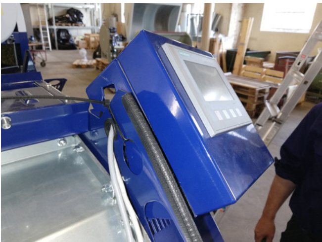
15 - the operator panel is detached from the blowers end plate, and secured as shown with a cable tie
