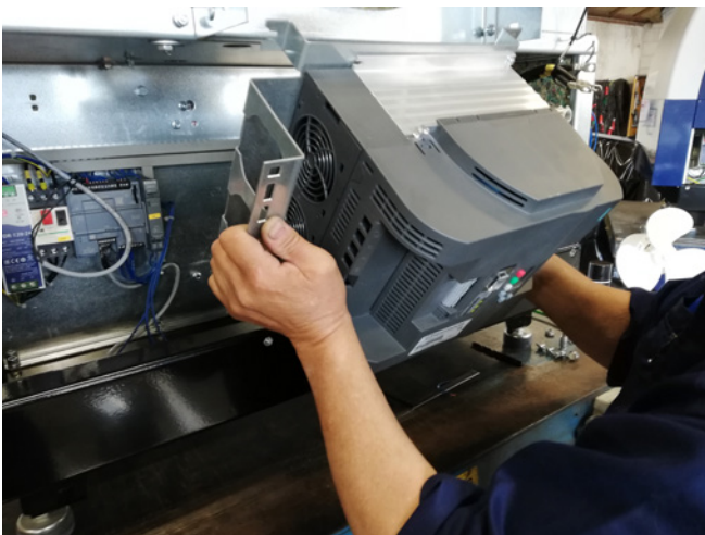
32 - refit the AC drive with the 4 screws
