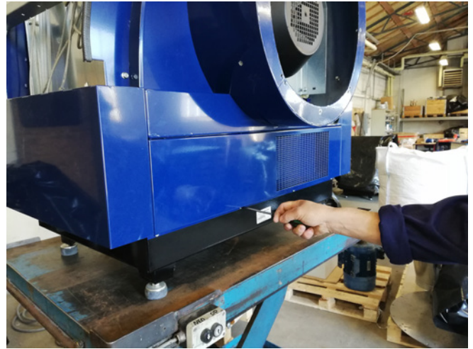
4 - remove the blue lower panel by removing 4 screws
