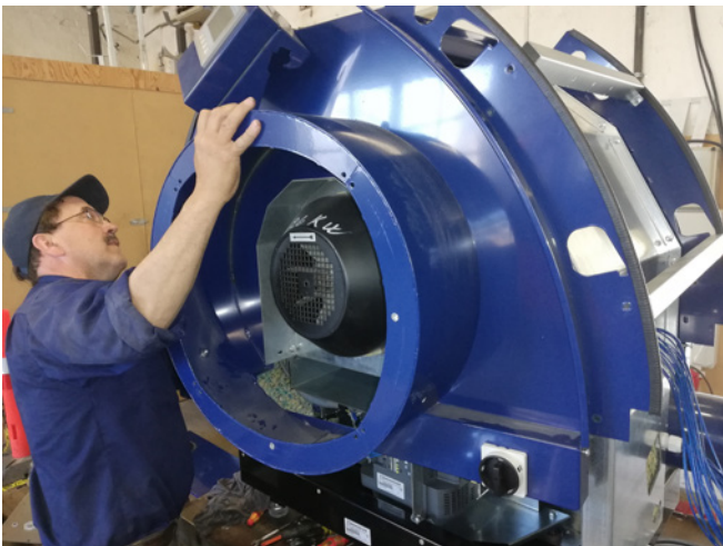
38 - refit the end plate, assuring that no cables are damaged, with the main switch in position OFF
