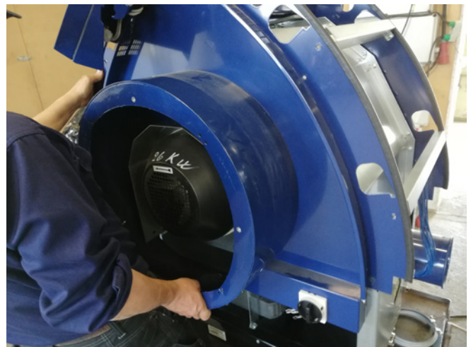
18 - grab the blowers end plate with both hands as shown, and lift slightly upward, and remove
