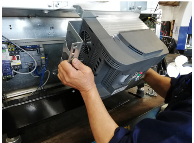
30 - push the AC drive with console to the right, tilt as indicated, and lift it out
