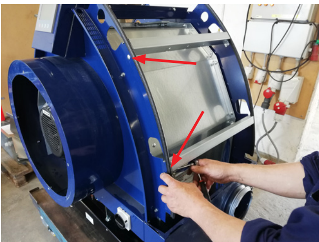
9 - remove 4 screws, 2 in each side
