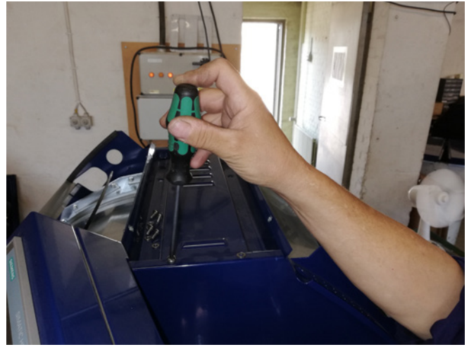
16 - loosen the blue back console by removing the 2 screws
