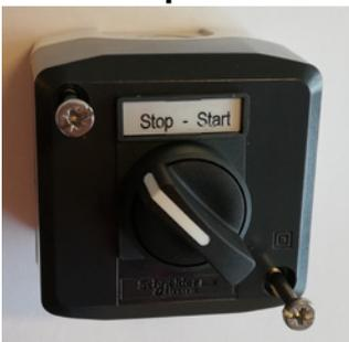
The external start / stop switch is connected in terminal block X30 between terminal 1 (+ 24VDC) and 3 (Digital Input 0), and a loop is installed between terminals 1 and 4.
