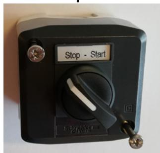
The external start / stop switch is connected in terminal block X30 between terminal 1 (+ 24VDC) and 3 (Digital Input 0), and a loop is installed between terminals 1 and 4.
