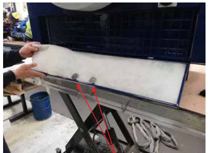
11 - the filter is accessible by opening the door, after which the filter can be cleaned or replaced. When the filter is inserted, ensure that the two slots are adjacent to the magnets
