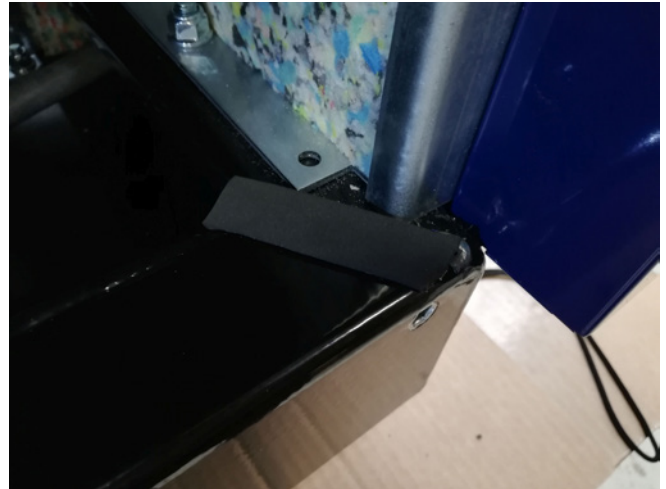
3 - cut off the foam strip as shown
