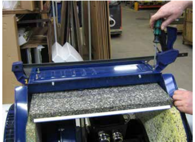
12 - reinstall the upper panel with the 4 screws. It can be necessary to press the side panels slightly, to align the screw holes.
