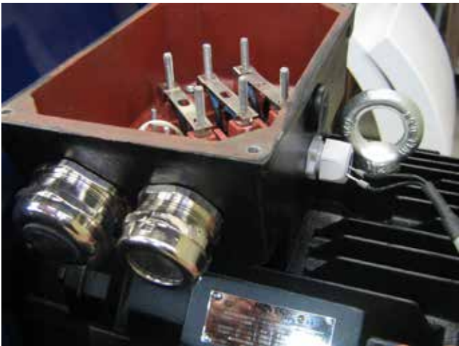
4 - the motor connection box lid is removed, and the thermistor cable is guided through the cable relief union as shown.
