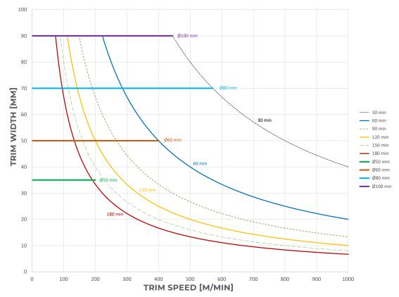
The diagram illustrates that transporting one 70 mm strip requires a Ø80 mm pipe, etc.
