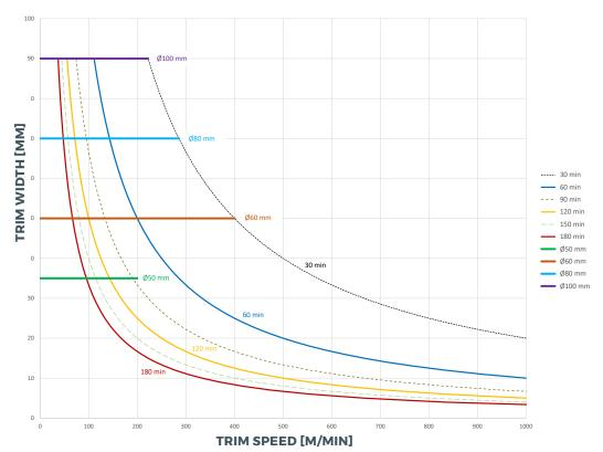
The diagram shows that to be able to suck two strips of 70 mm, you need a Ø80mm pipe, etc.
