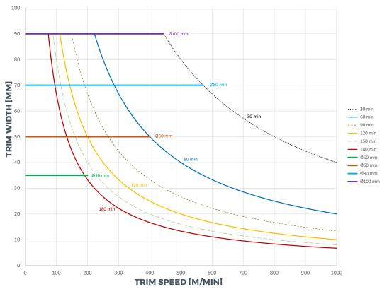
The diagram shows that to be able to suck one strip of 70 mm, you need a Ø80mm pipe, etc.
