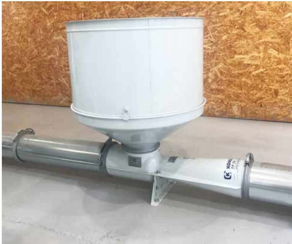
The TF Injector with hopper and mounted feeder unit
