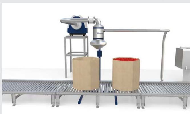
The Kongskilde systems can handle components from 10-50 mm in diameter. More than 250,000 units may be moved per hour.
