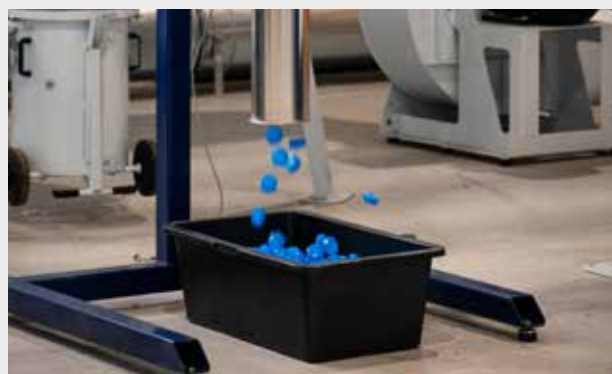
The finished components may be gently conveyed from storage to be delivered in apportioned volumes for packaging.
