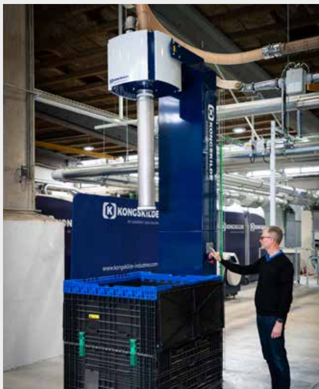
Finished components are conveyed from stocking area to the production or packaging areas by means of the Component Pick-up Unit - CPU.
