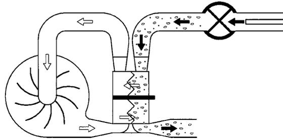
The rotor of the Multiseparator is in two parts, separated by a perforated screen the whole revolving at a low speed. On the upper, or inlet, side, the conveying air passes through the perforated screen to the blower intake, whilst waste material is retained.
