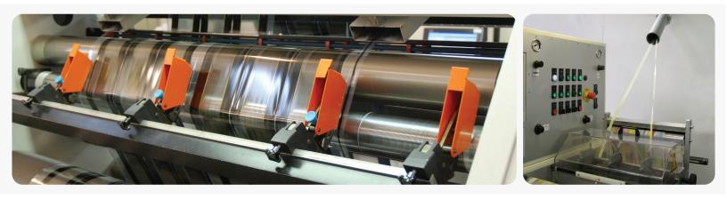
Kongskilde waste extraction systems efficiently handle trims from film and foil production (cast lines) and converting machines (slitters/re-winders). The patented ITF Venturi, capable of conveying endless trim at speeds exceeding 1000m/min\*, is a proven solution for various applications.
