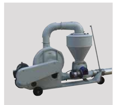
Suction blower used for conveying from and to multiple destinations.
