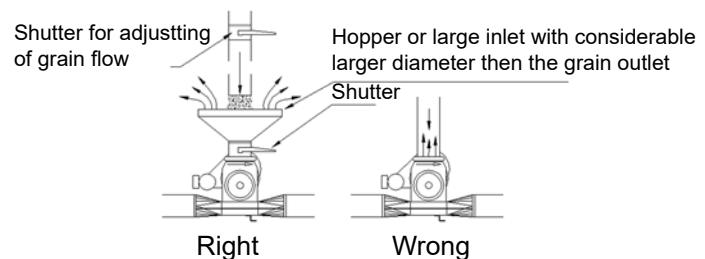
NOTE: If the rotary valve is dismantled, make sure that it is assembled correctly again! - The top part/rotary valve and bottom part/outlet can be assembled inversely!
