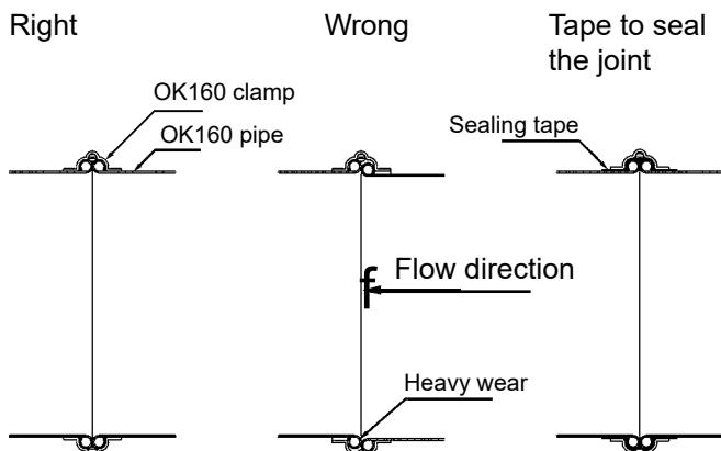
Do not rely on centering the pipe with the clamps alone. The clamp is designed for pressing the OK-pipe ends very hard together in order to ensure a very high tightness. This causes the friction between the pipes to become so high, that the clamp is unable to center the pipes. Check gap between clamp and pipe to ensure it is similar on both sides. Check the pipeline visually to secure a straight line.
