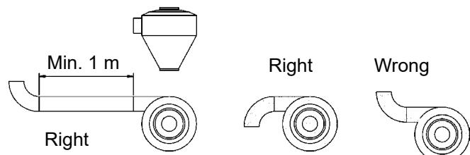
Do not install a bend turning in the opposite direction of the cyclone right in front of the entry. If this is done, the effect of the cyclone is more or less neutralized.
