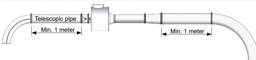
Do not extend the ITF's outlet pipe with the same pipe diameter, but increase the diameter of the pipe in accordance with tables B and C. Do not use a transition immediately before a bend.
