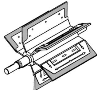
The life of the paddles will depend on the type of materials conveyed through the valve. As the paddles are subject to increasing wear, more air will pass the rotor. This leakage will make it more difficult for the material to fall down into the valve and, accordingly, reduce the capacity. When the capacity has decreased unacceptably, replace the paddles.
