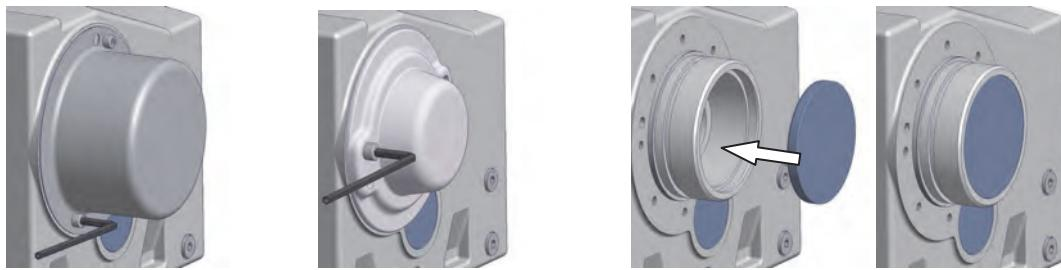
Figure 3-12: Fitting the covers, Option SH, Option H, and Option H66
