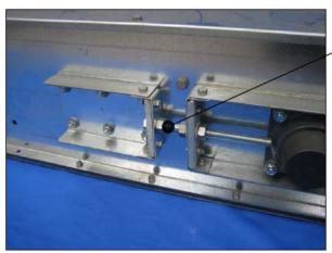
Regular adjustment of the chain tension is carried out with use of the chain tensioning screw of the conveyor.
