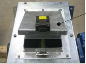
Install the safety switch that is triggered on overfilling, check its operability.
