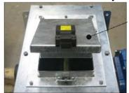
In addition, the chain conveyor should be equipped with a main power switch locked with a key. This switch is to be used to shutdown the conveyor before dismantling its covers to prevent the machine from unintentional starting up. The safety switch must be placed on the conveyor or within its working area.
