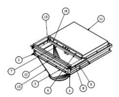
The intermediate outlet is made up of the frame, the gate valve of the PE board combined with a pneumatic cylinder. To mount the outlet it is necessary to make an opening in the conveyer bottom at the location of the outlet and then attach the outlet frame to the conveyer frame and bottom plate by means of bolts.
