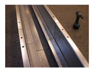
The conveyor has to be supported at both ends, and with a max. distance of 4.5 meters between the supports. It is important that the support of the drive section is making sure that the drive section is not out of angle, because of the weight of the gearbox and motor
