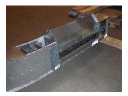
The horizontal section before the angle section has a plate for the return chain which goes into the angle section.
