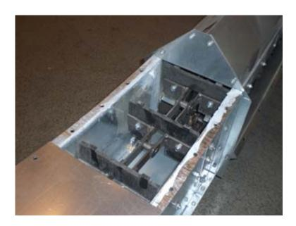
Check that all connections of the bottom plates are facing each other to make sure that there are no edges the plastic paddles may encounter. Return rails have also to be checked and adjusted if necessary. Loosen the bolts and move the nearest rails up or down if necessary
