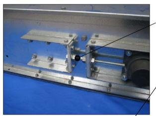
Regular adjustment of the chain tension is carried out with use of the chain tensioning screw of the conveyor.
