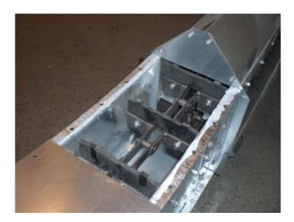
Check that all connections of the bottom plates are facing each other to make sure that there are no edges the plastic paddles may encounter. Return rails have also to be checked and adjusted if necessary. Loosen the bolts and move the nearest rails up or down if necessary
