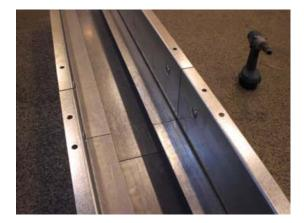
The conveyor has to be supported at both ends, and with a max. distance of 4.5 meters between the supports. It is important that the support of the drive section is making sure that the drive section is not out of angle, because of the weight of the gearbox and motor
