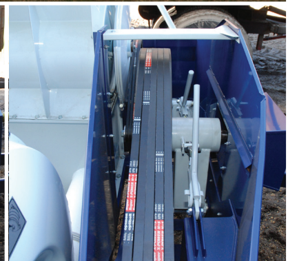
The belts can be tightened without using tools.
