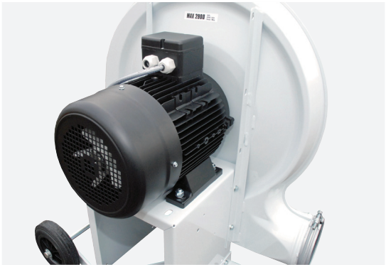
The motor directly drives the blower rotor.
