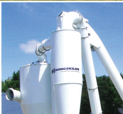
Fan guard reduces wear, removing abrasive material before it enters the fan.
