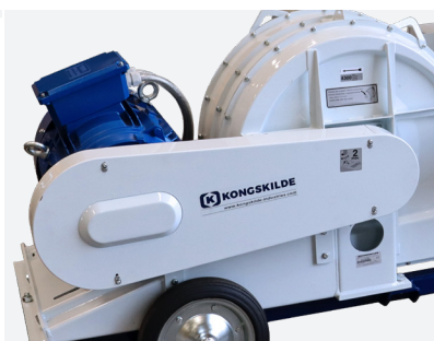
Belt transmission protects drive of both blower and cell wheel.
