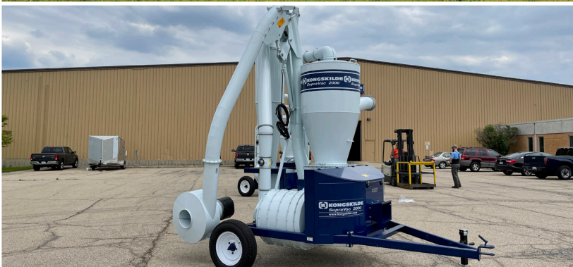
SupraVac 2000 hydraulically folded into transport position.
