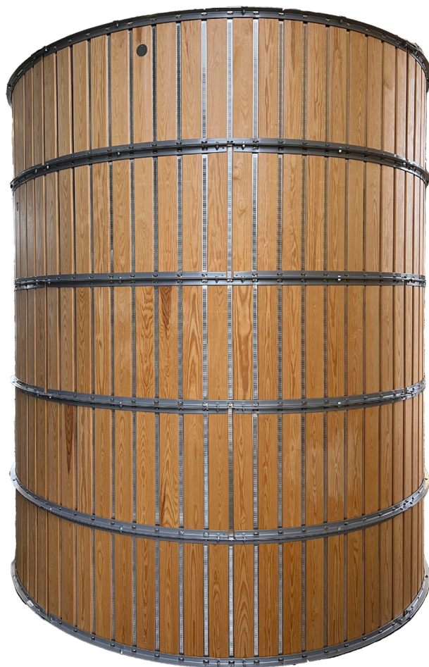
The silos are built of modular sections made of wood and aluminium fitted together with angle iron hoops.
