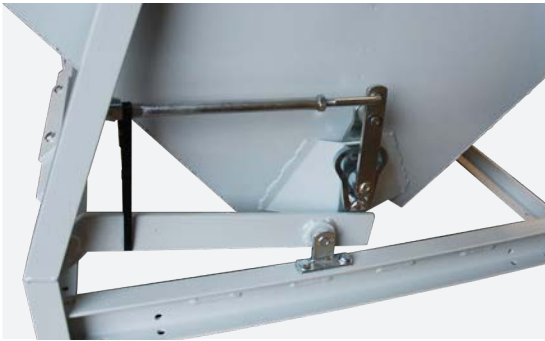
KA batch weigher trip mechanism.
