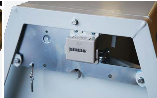
KA batch weigher mechanical counter.
