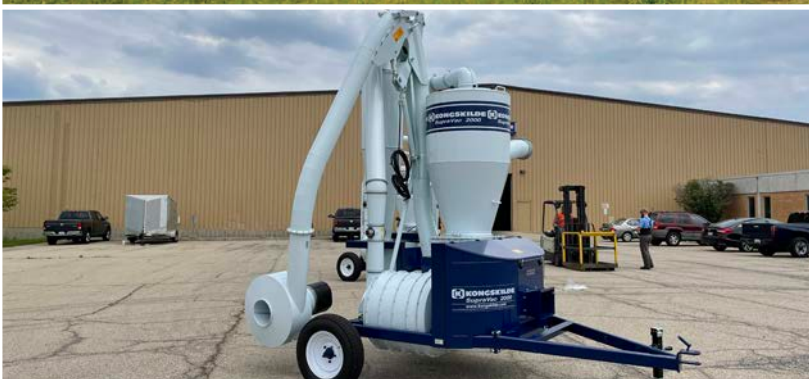
SupraVac 2000 hydraulically folded into transport position.
