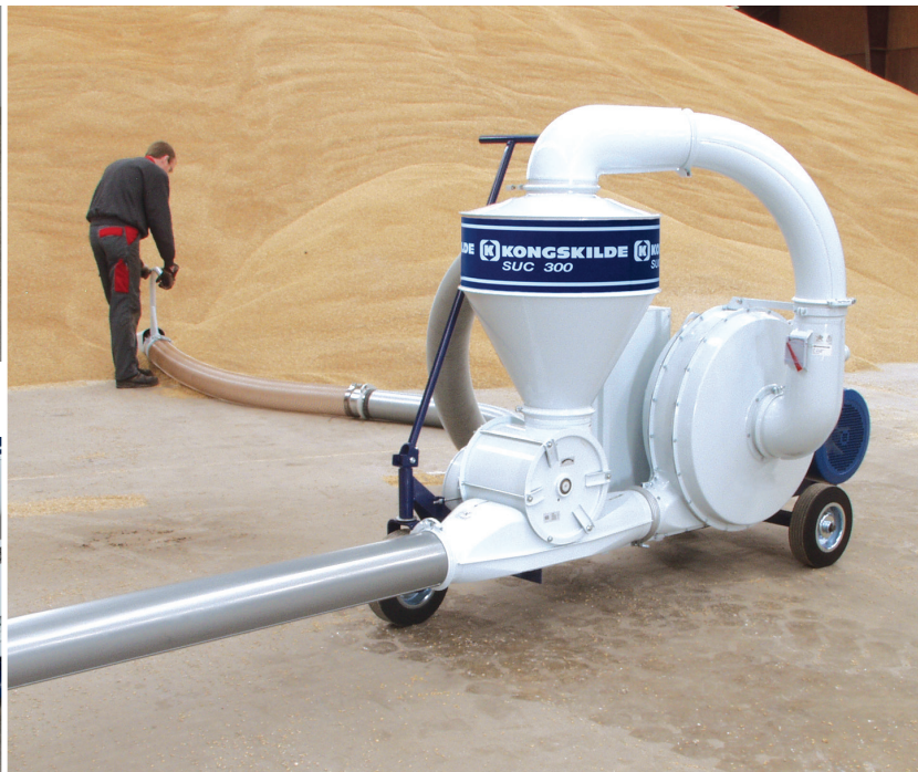
SUC 300 suction blower being used to convey grain.
