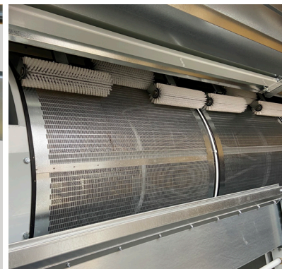
The cleaning brushes are mounted on a spring loaded arm for efficient even load on the outer screens
