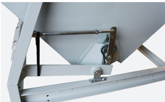
KA batch weigher trip mechanism.
