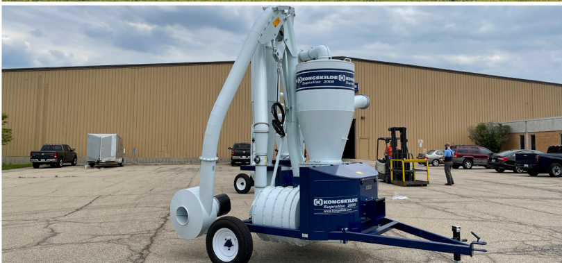
SupraVac 2000 hydraulically folded into transport position.
