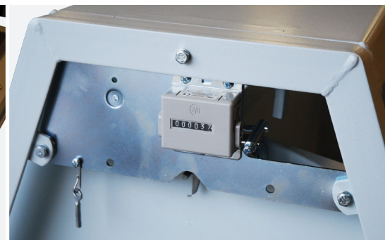
KA batch weigher mechanical counter.
