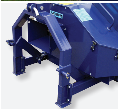
Mounting frame for attachment to three-point hitch.
