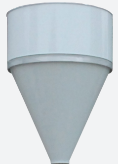
Cyclone for discharge of dust.
