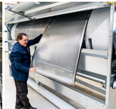
A quick-release system makes it easy and fast to change screens and make ready for the next crop
