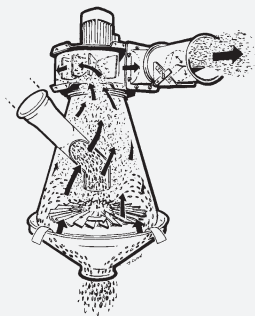
KF 40 mode of operation.
