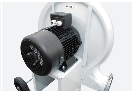
The motor directly drives the blower rotor.
