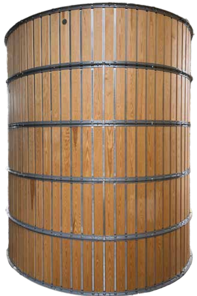
The silos are built of modular sections made of wood and aluminium fitted together with angle iron hoops.
