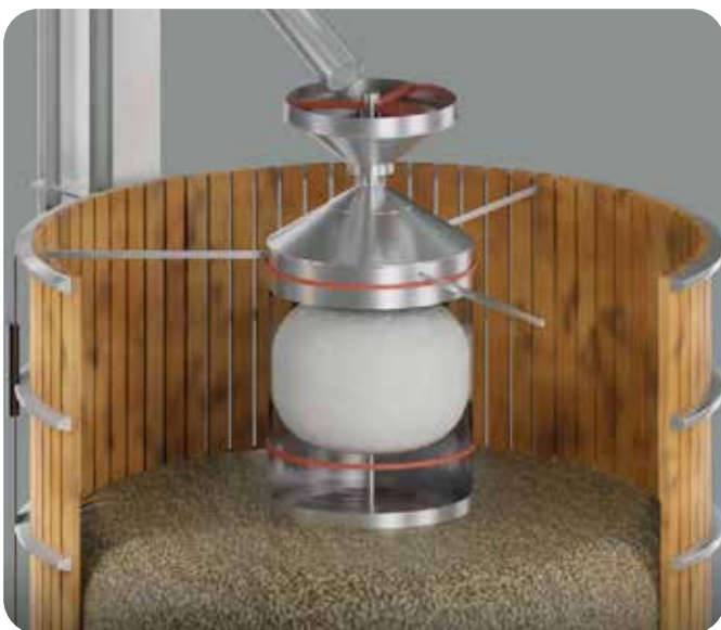
The canvas bag is open at the bottom, and the upgoing airstream will press the canvas against the inside of the ventilation pipe and prevent the air from passing by the valve.
