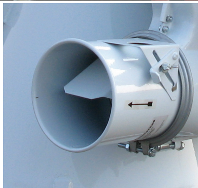
Air regulator for adjustment of the suction power of the aspirator blower.
