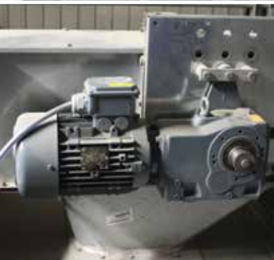
Bevel gear motor with high efficiency.
