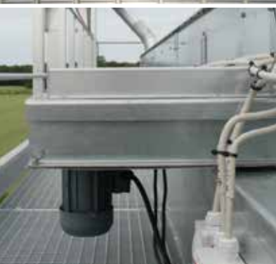
Motorized intermediate outlet.
