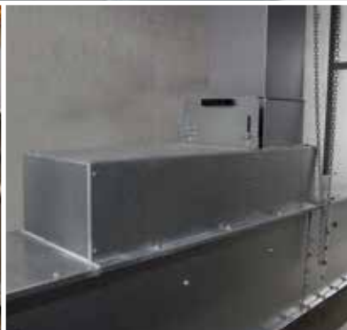
Intermediate Inlet with capacity control.
