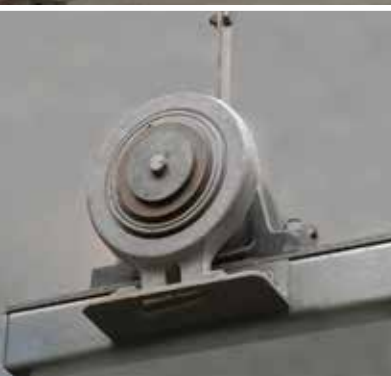
The back stop prevents the elevator belt from running backwards (optional).
