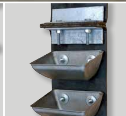
Assembly of belt - mounting of buckets with self-locking nuts.
