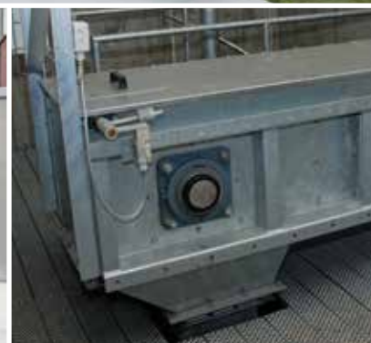
Drive section with outlet and overflow.
