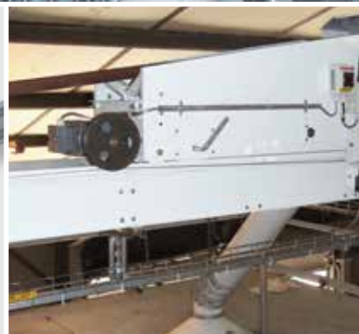
Motorized discharge unit for BCB 45.
