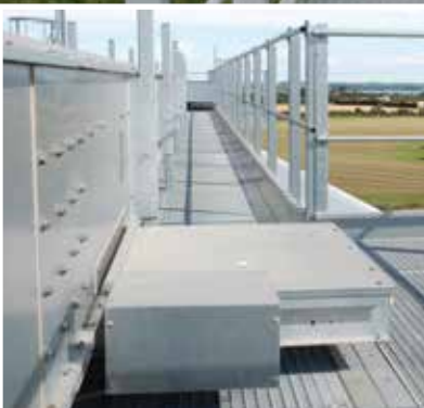
Intermediate outlet fitted in the conveyor base. Operated manually or electrically.
