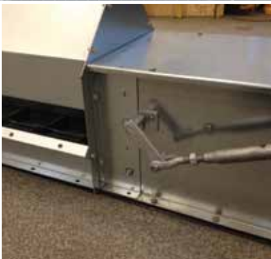
Extension with side inlet and capacity control.
