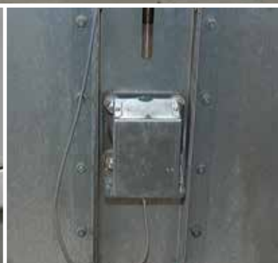
The speed sensor signals when the bucket belt stops (optional).
