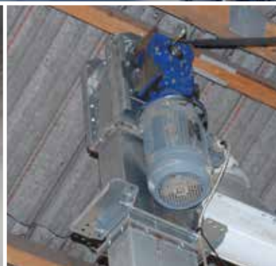
Elevator head with gear motor.
