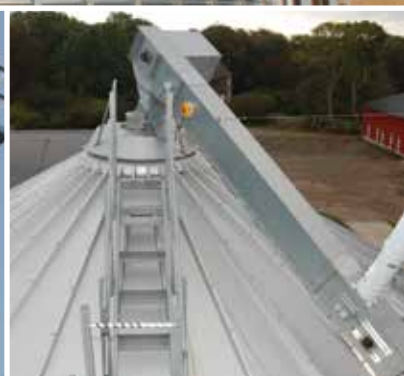
Chain conveyor mounted on silo roof. Rain cover for bevel gear motor.
