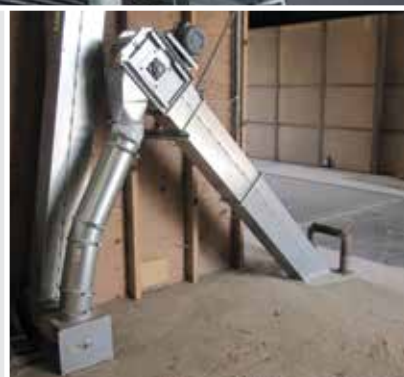
Chain elevator from the grain pit delivers the grain to the flexible foot on the next elevator.
