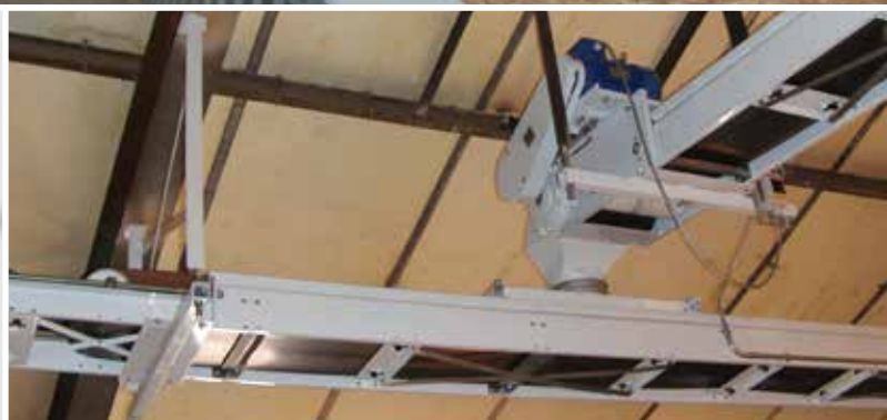
Solution with two belts fitted at a 90° angle. The lower conveyor belt can move lengthwise.
