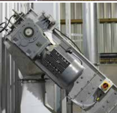
Bevel gear motor provides compact solution.
