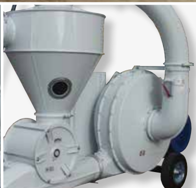
SUC 300E with automatic air regulation.
