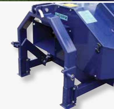
Three-point attachment to tractor lift.
