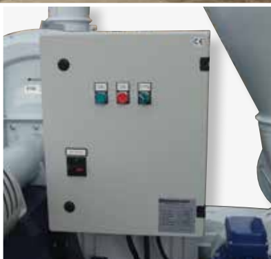
Control cabinet for automatic starting/stopping the motor.
