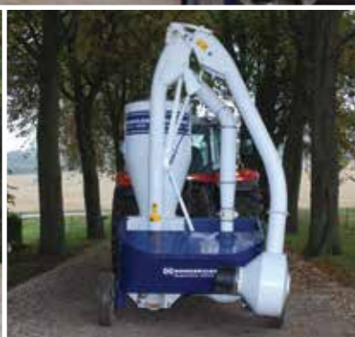
Loading equipment hydraulically folded to transport position.
