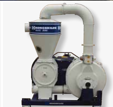
Three-stage blower on SUC 500T provides high pressure for grain conveying.
