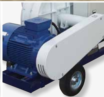
Belt transmission protects drive of both blower and rotary valve.
