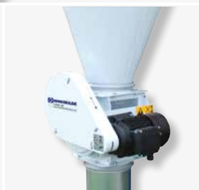
CAE 20 rotary valve mounted below the cyclone in a pure suction installation.
