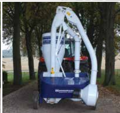
Loading equipment hydraulically folded to transport position.
