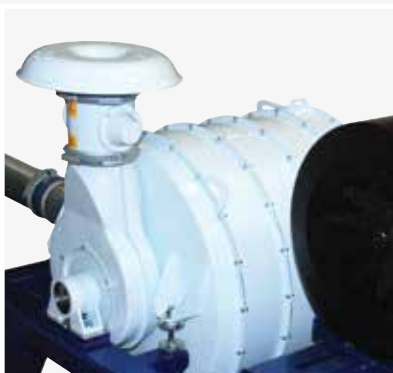
Automatic air control on TRL 1000. Damper closes automatically during startup.
